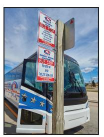
If you will need to use a wheelchair lift, park the vehicle where the lift can be used and accessed. You need both a clear area for the wheelchair lift to deploy and a clear approach area to load the passenger onto the lift.
